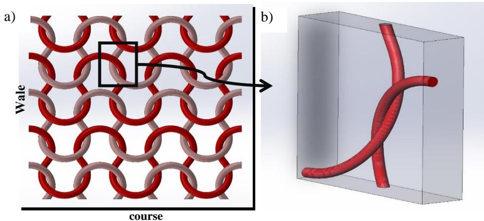
Fig. 1. Knitted fabric geometry (a) unit cell of the model used for simulation (b)
