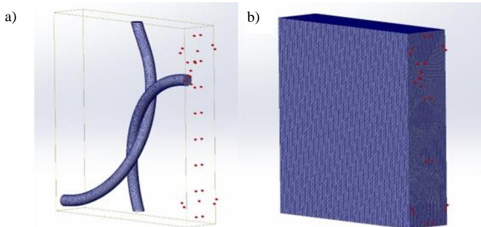
Fig. 2. Mesh in yarn (a) and mesh in unit cell (b)
